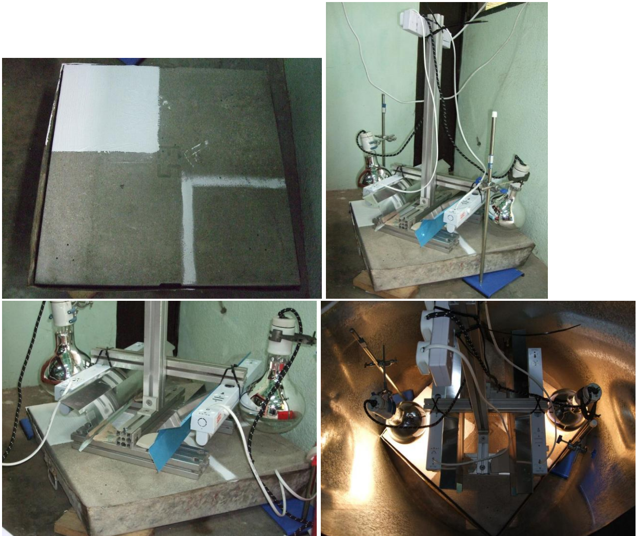
Fig.1. Accelerated ageing system.
