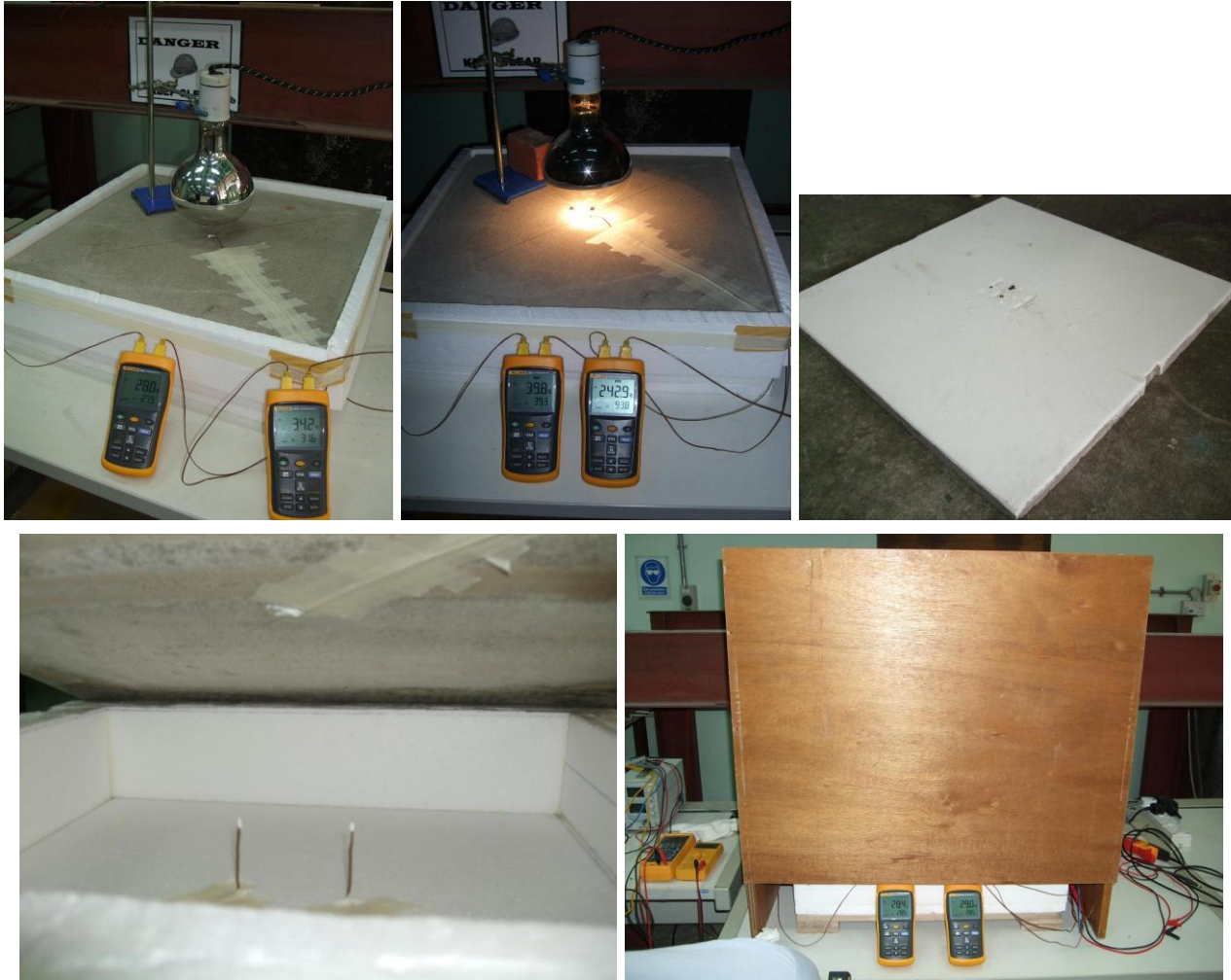
Fig.2. Thermal insulation testing system.
